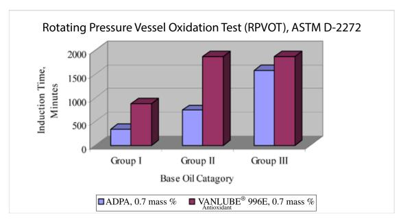
**Figure 2.** Rust inhibitor (**VANLUBE RI-A** Lubricant Additive, 0.05 mass %) was added to all test oils. ADPA is acronym for alkylated diphenylamine. The ADPA that was used for this study consisted of a mixture of butylated/octylated DPA components.
