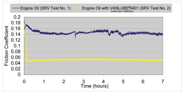
**Figure 1.** Test Parameters: ball on disk; 120N; 40 Hz; 4.00 mm stroke; 7 hours. The engine oil is 5W-30 grade containing 0.05 mass percent of phosphorus.
