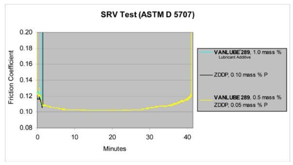
**Figure 5.** Test Parameters: 25°C; 50 N break-in load; 1000 N test load; 50 HZ; 1.00 mm stroke. Experiments ran until failure as indicated by a large and sudden increase in the friction coefficients
