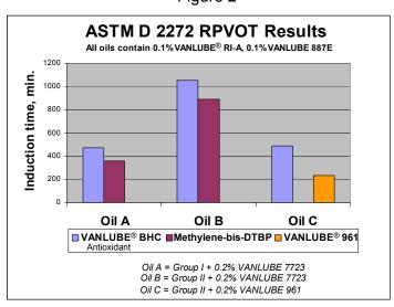
VANLUBE SL and VANLUBE 961 are alkylated diphenyamines; VANLUBE 7723 is methylene-bis-dibutyl-dithiocarbamate
