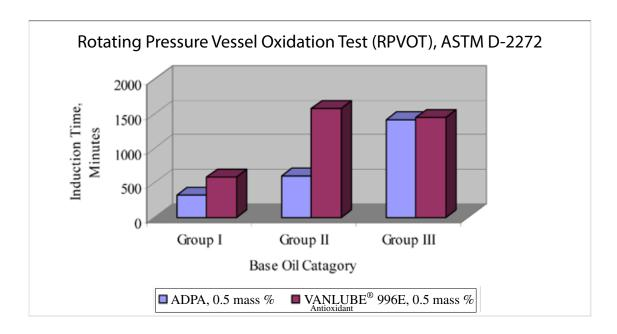
**Figure 1.** Rust inhibitor (**VANLUBE® RI-A** Lubricant Additive, 0.05 mass %) was added to all test oils. ADPA is acronym for alkylated diphenylamine. The ADPA that was used for this study consisted of a mixture of butylated/octylated DPA components.
