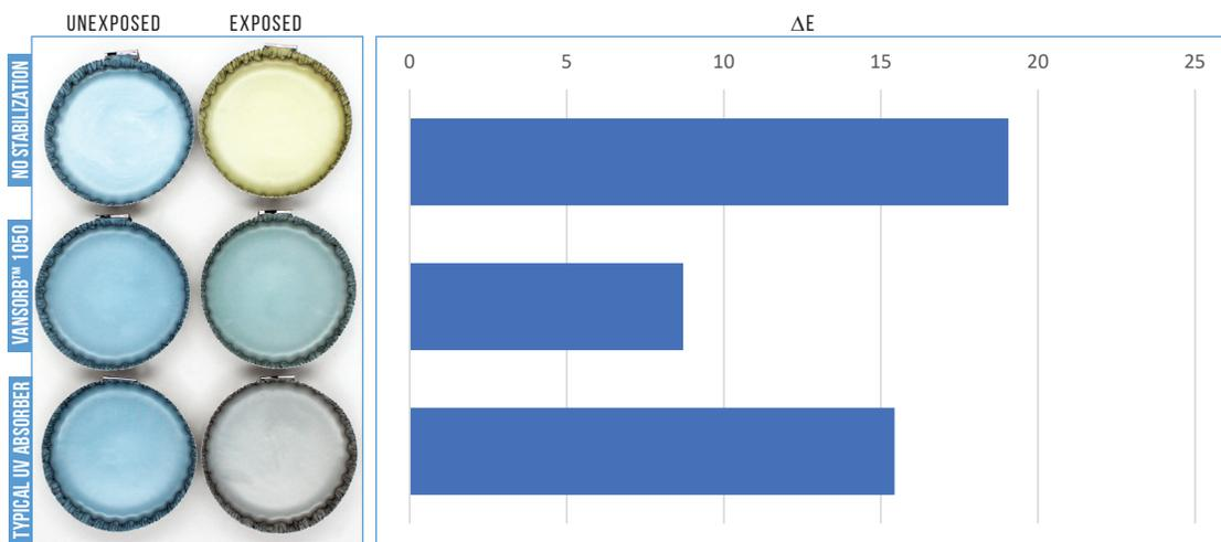
Scented paraffin wax candle formulation containing 0.2% stabilization in a light box with continuing exposure to black light for 72 hours.
