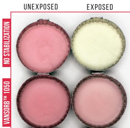
Scented 70/30 paraffin/soy wax candle formulation containing 0.2% stabilization in a light box with continuing exposure to black light for 72 hours.
