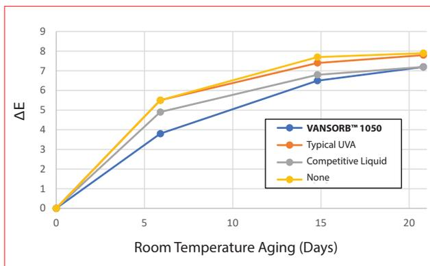
Scented soy wax candle formulation containing 0.2% stabilization aging at room temperature.
