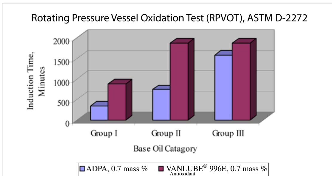
**Figure 2.** Rust inhibitor (**VANLUBE RI-A** Lubricant Additive, 0.05 mass %) was added to all test oils. ADPA is acronym for alkylated diphenylamine. The ADPA that was used for this study consisted of a mixture of butylated/octylated DPA components.
