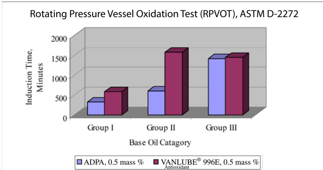
**Figure 1.** Rust inhibitor (**VANLUBE® RI-A** Lubricant Additive, 0.05 mass %) was added to all test oils. ADPA is acronym for alkylated diphenylamine. The ADPA that was used for this study consisted of a mixture of butylated/octylated DPA components.
